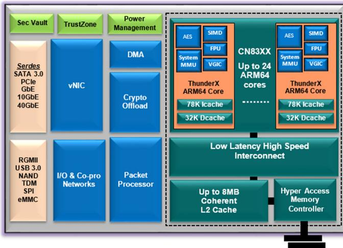
Figure 1. The Cavium OCTEON TX ARMv8 SoC family.
