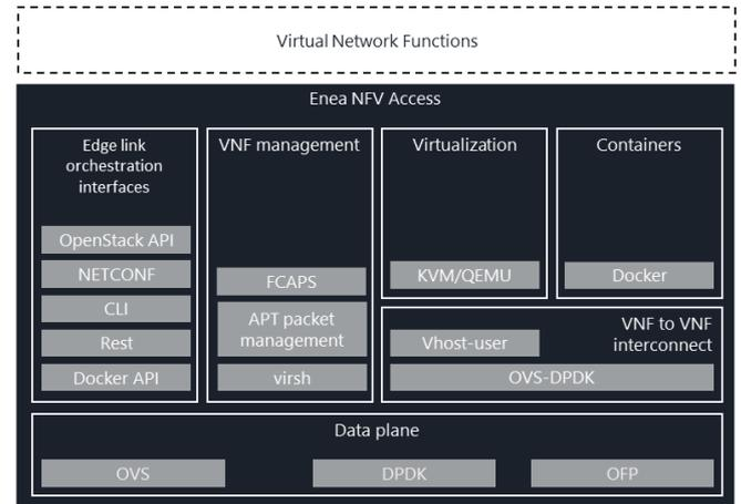
Figure 2. The Enea NFV Access software platform.
